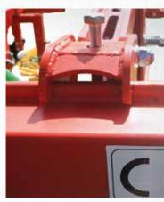
The machine is equipped with three-point linkage cat. II, with supporting wheels (adjustable height and spacing)
