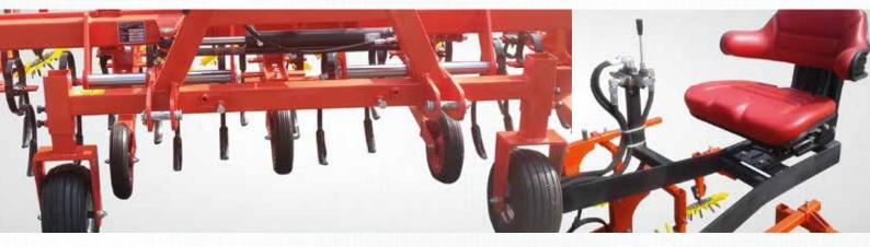
The working sections of the machine are equipped with a mechanism for quick change of working depth, through a knob that extends or slides the supporting wheel into the machine body. The working section is equipped with 5 spring tines \$ 32x10 with a straight coulter or a duck foot. There is also the possibility of ridges mounting. The machine is equipped with a rapid displacement system of working sections, which simplifies working width configuration for a given crop.
